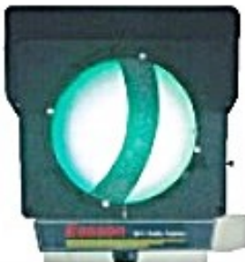
Reject Weld Area; High-lighted on Vulcan's Esscon® Profile projector.
